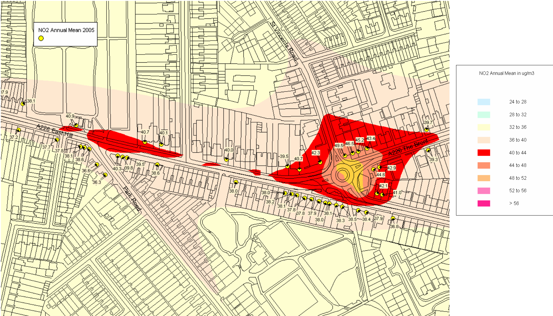
Figure 14 2005 NO 2 Annual Mean Junction 3 & 4: A226 East Hill/Park Road and A226 The Brent/Watling Street
